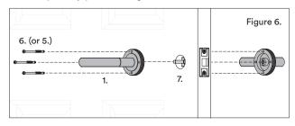
† For Helsinki lever unscrew end cap to remove and fit rose.
